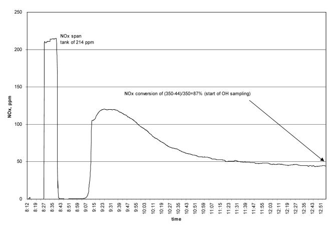
Figure 2. NO<sub>x</sub> concentration vs. time (hours:minutes) measured at SCR reactor outlet for Test B1.
