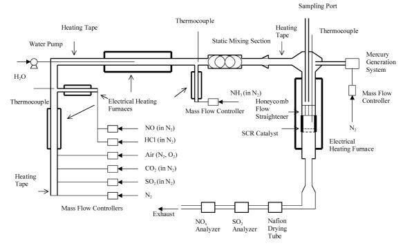
Figure 1. SCR reactor system.
