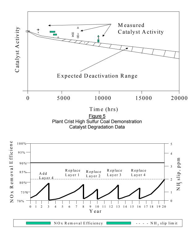
Figure 6 Typical Catalyst Management for Cyclone Boiler 100% ash Recircualtion
