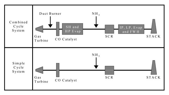
Figure 2 Gas Turbine SCR Arrangements
