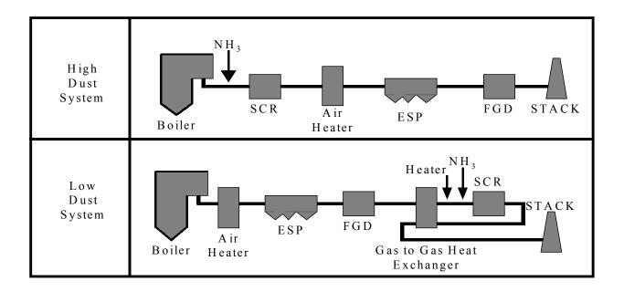
Figure 3 Boiler SCR Arrangements
