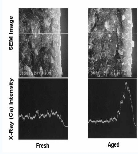
Image 1: CaO Deposition and CaSO4 Masking Images captured by a scanning electron microscope (SEM)
